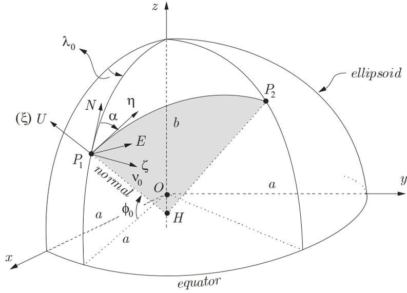
Figure 6: Rotated local coordinate system  $\zeta, \eta, \xi$
