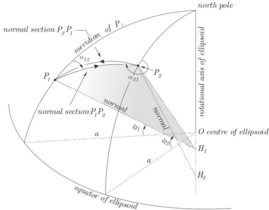
Figure 3: Normal section curves between  $P_1$  and  $P_2$  on the ellipsoid
