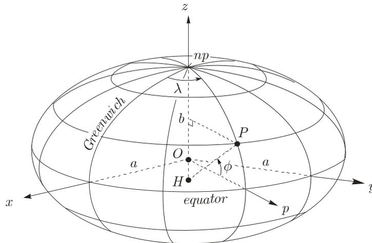
Figure 1: The reference ellipsoid
