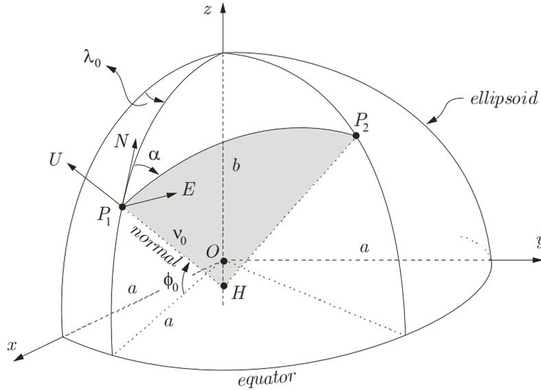
Figure 5: Normal section plane between  $P_1$  and  $P_2$  on the ellipsoid
